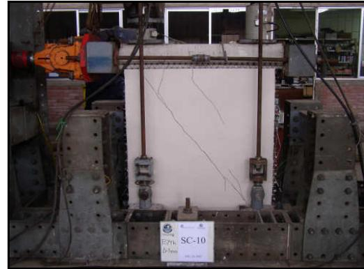
**Figure 7** Set up and for reinforced panels.
