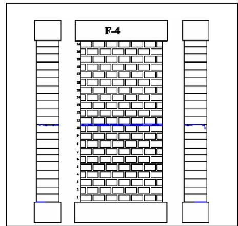
**Figure 17.** Crack pattern F-4
