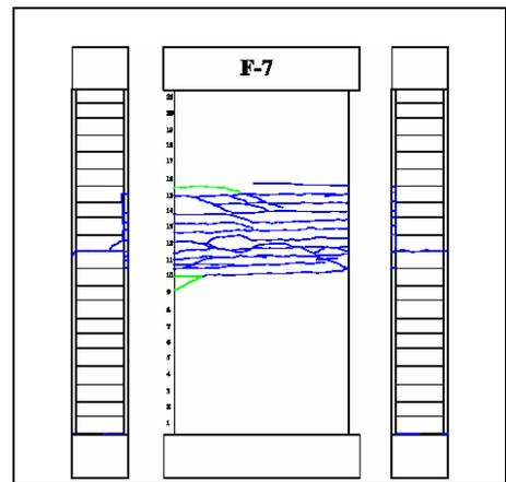
**Figure 21. Crack pattern F-7.**
