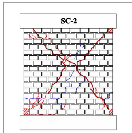
**Figure 10.** Crack pattern SC-2
