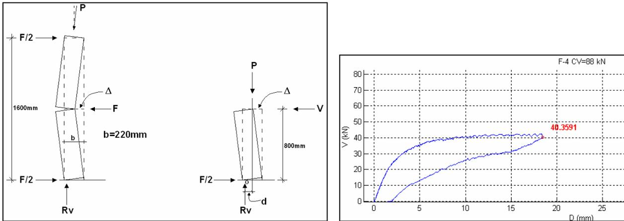
**Figure 24.** Out-of-plane response of plain walls with vertical load and F-D curve for F-4.
