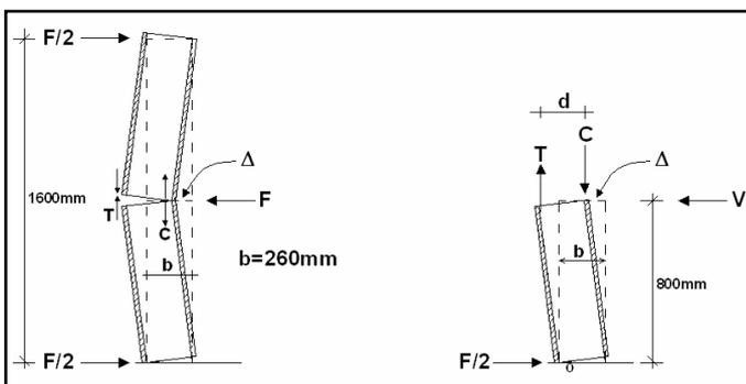
**Figure 25.** Out-of-plane response of panels reinforced with polymer grid, without vertical load.
