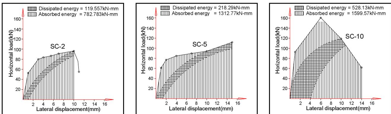
Figure 15 Computation of absorbed and dissipated energy for three types of panels.
