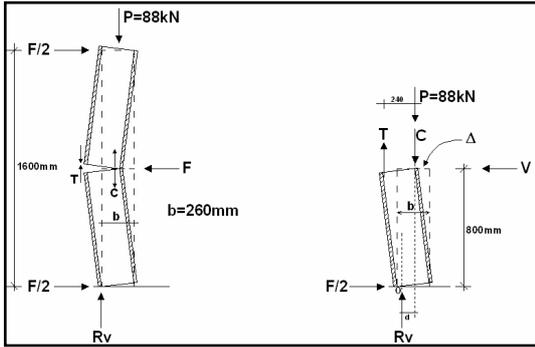
**Figure 26.** Out-of-plane response of reinforced panels with additional vertical load.
