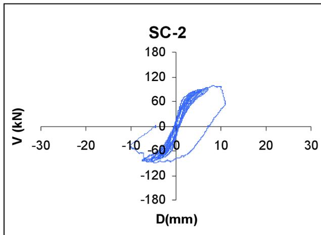
**Figure 9.** SC-2 - Force - displacement curve
