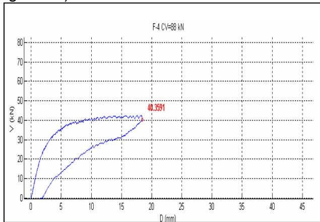
**Figure 16.** F-4 Force-Displacement curve
