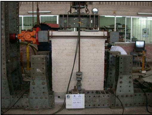
**Figure 6.** Set up for non reinforced panels
