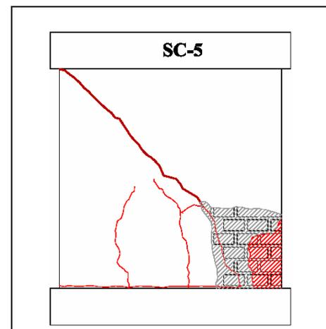
**Figure 12.** Crack pattern SC-5.
