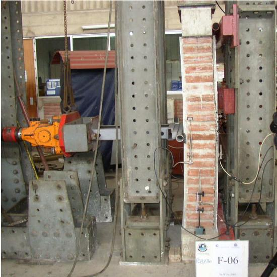
**Figure 8.** Experimental set up for flexural panels.
