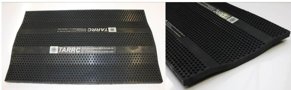
Fig. 6 – TARRC’s horizontal joints used in the laboratory structural tests at the University of Padua
